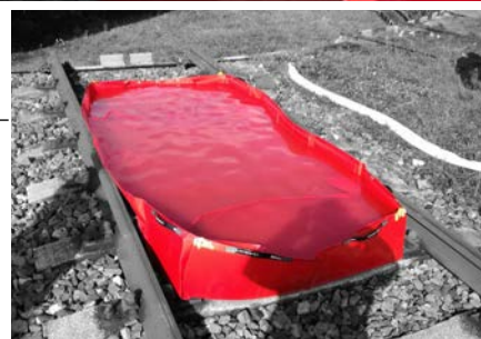
There are two ways to place the tank under a train or other track vehicle: across the rails or along them into the inner space between the rails. Both ways passed very strict testing.
