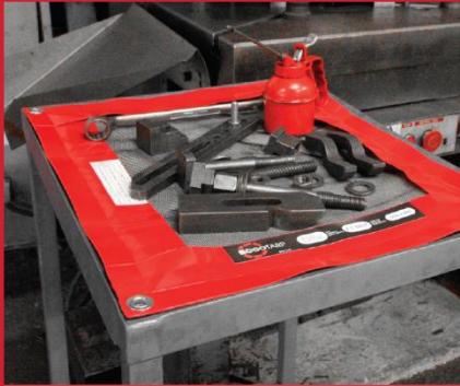
Folding drip collection tray with exchangeable absorbent lining
